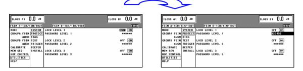
Execute the calibrations from the menu UTILITIES/CALIB/ALL. The generator should be in a warmed-up condition (at least 30 minutes switched on). After the calibration all errors will disappear.
